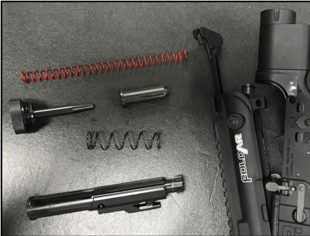
Action and recoil components of the Dead Foot Arms Modified Cycle System.
